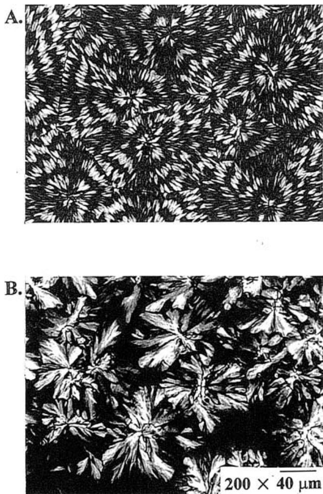
Fig. 10 Reversibility of the ring bands in PCL spherulites in the PCL/PBzMA blend (70/30): A slowly cooled from above the lower critical solubility temperatures (LCST) returning to phase homogeneity and subsequent ring bands; B quenched from above the LCST showing the absence of ring bands owing to a phase-separated state
